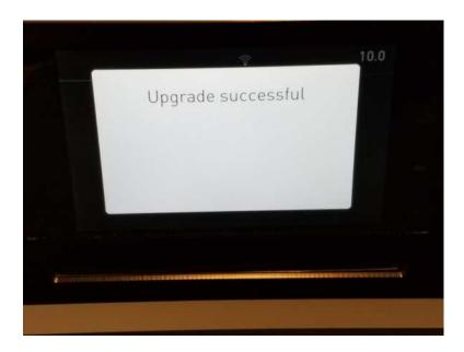
r. When 9 minutes has elapsed the display should show the Upgrade successful message. If you get a message that says Upgrade Failed you will need to either contact customer support or download sfupdate and run the USB update to recover the No519.
