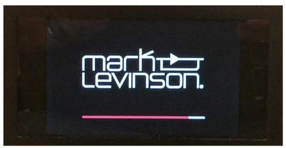
p. After 8 ½ minutes have passed the Mark Levinson splash screen is shown on the display and the Standby LED remains flashing quickly.
