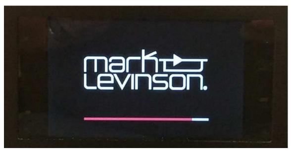
k. Once 2 ½ minutes have passed the LED is still flashing quickly and the display has turned on and is showing the Mark Levinson splash screen.
