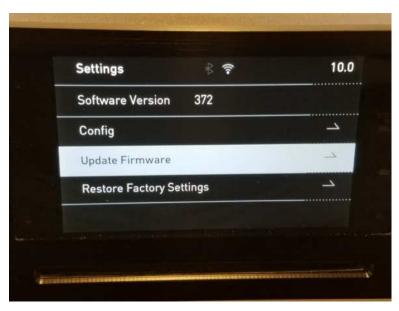
e. Adjust volume knob clockwise to highlight Update Firmware, then press the Select button on the front panel.
