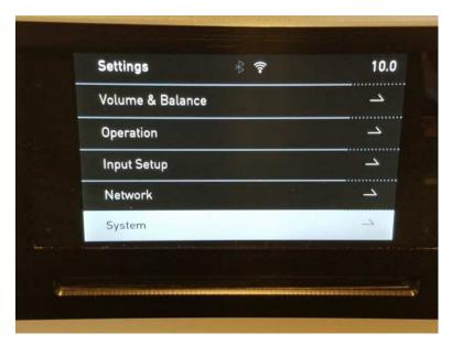
d. Adjust volume knob clockwise to highlight System, then press the Select button on the front panel.
