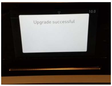
r. When 9 minutes has elapsed the display should show the Upgrade successful message. If you get a message that says Upgrade Failed repeat the Software upgrade procedure from the beginning.
