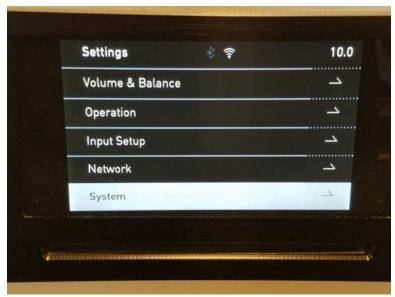
d. Adjust volume knob clockwise to highlight System, then press the Select button
