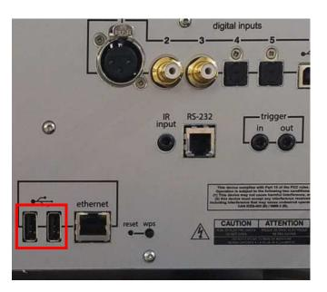
f. When you see the 'Update firmware' screen, plug the USB Thumb drive with the sfupdate file into one of the USB-A connectors on the rear panel of the No519
