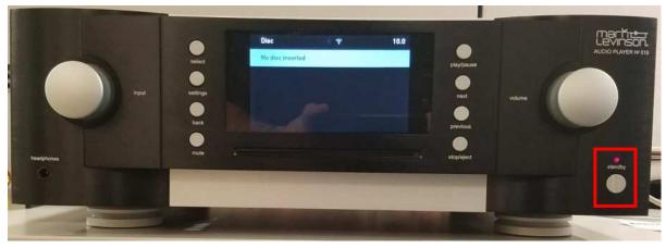
j. After 1 minute has elapsed the display will turn off and the Standby LED will start flashing quickly.
