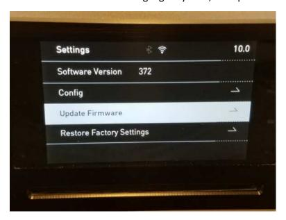
e. Adjust volume knob clockwise to highlight Update Firmware, then press the Select button.
